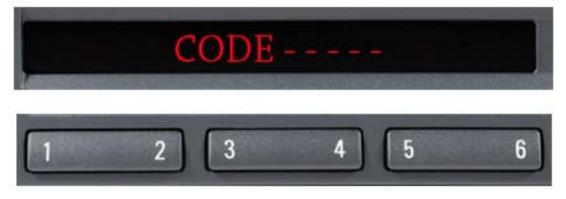
Use the station preset keys 1-6 (figure 1 # 7) to enter the 5 digit code. For example, if the code is 63251, press 6 key followed by the 3,2,5 & 1 key.
